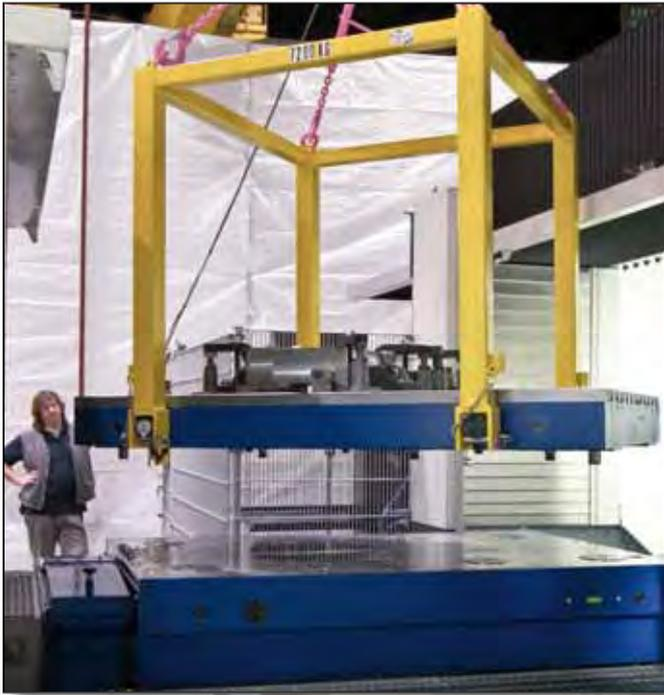
*Pallet changer and zero-point clamping systems* for efficient production through parallel set-up and processing times.
