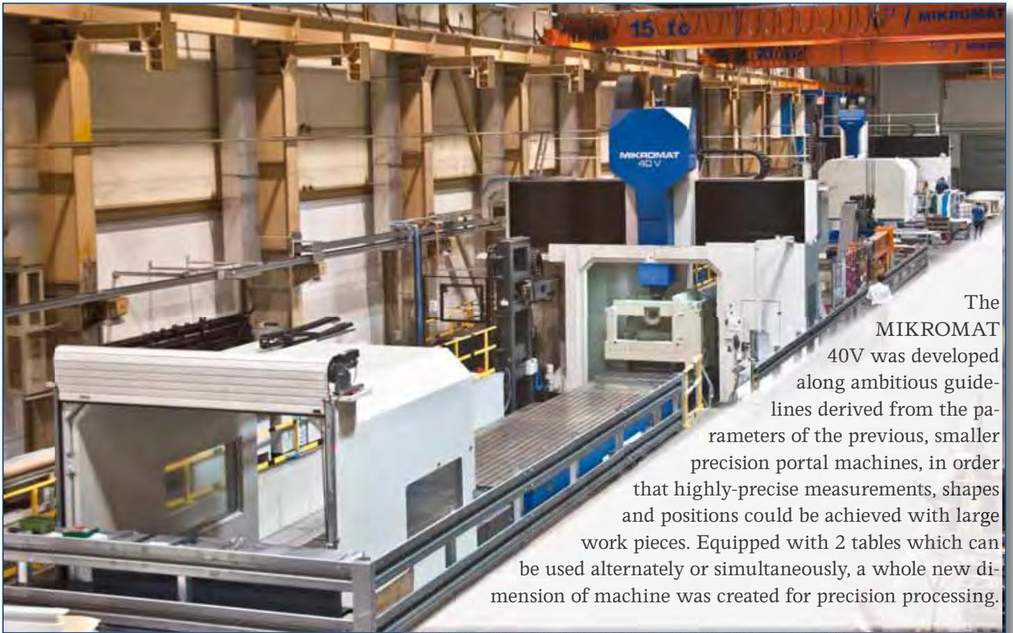
The MIKROMAT 40V was developed along ambitious guidelines derived from the parameters of the previous, smaller precision portal machines, in order that highly-precise measurements, shapes and positions could be achieved with large work pieces. Equipped with 2 tables which can be used alternately or simultaneously, a whole new dimension of machine was created for precision processing.
