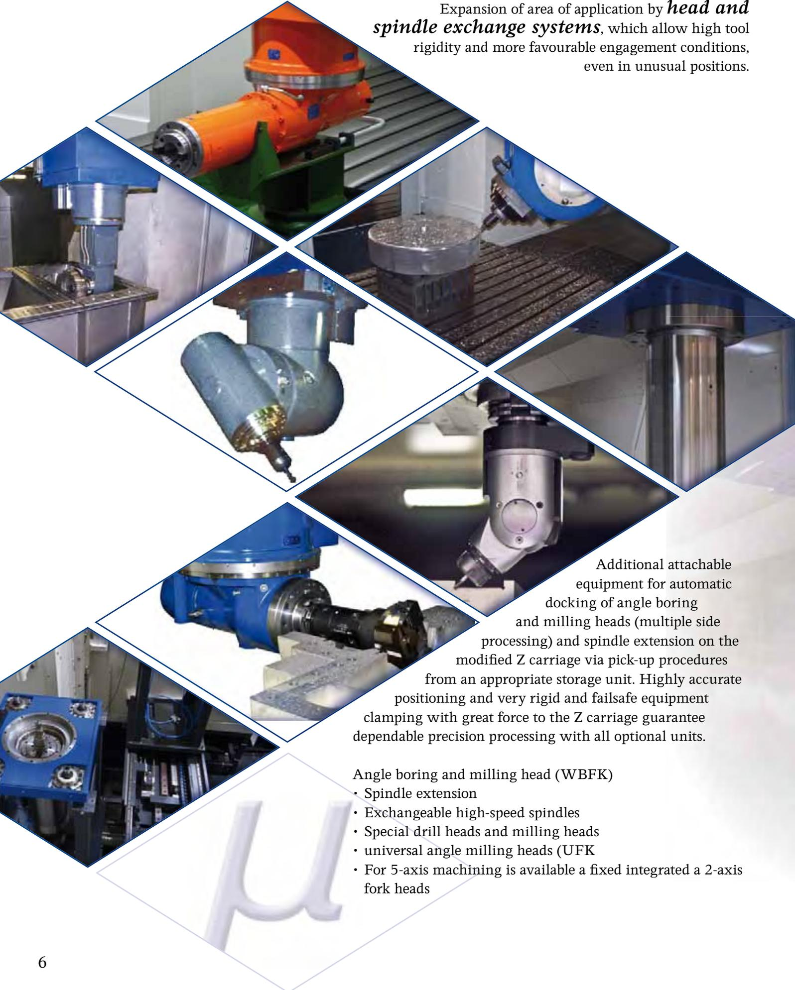
Additional attachable equipment for automatic docking of angle boring and milling heads (multiple side processing) and spindle extension on the modified Z carriage via pick-up procedures from an appropriate storage unit. Highly accurate positioning and very rigid and failsafe equipment clamping with great force to the Z carriage guarantee dependable precision processing with all optional units.
