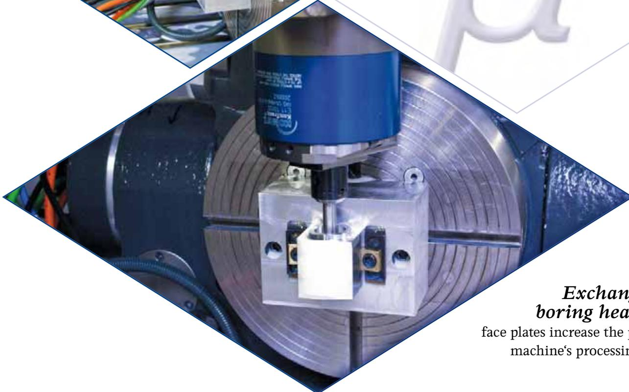
***Exchangeable boring heads*** with face plates increase the precision machine's processing range.
