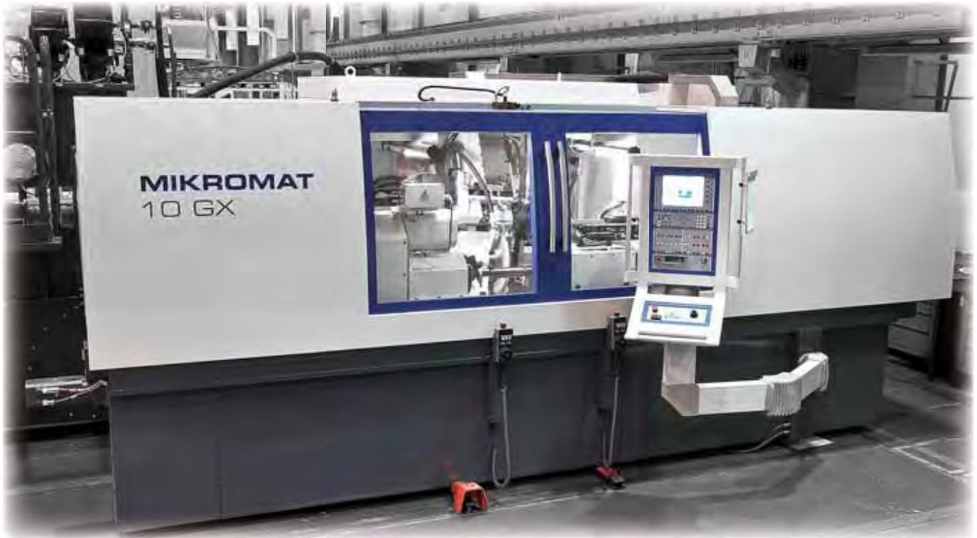
*The rotational form and thread grinding machines* are characterised by their high production quality, performance, universality and comfort. Due to the technical parameters, the machines can be used efficiently for the intensive and finishing grinding of various work piece geometries, with high effectiveness and the highest level of precision.
