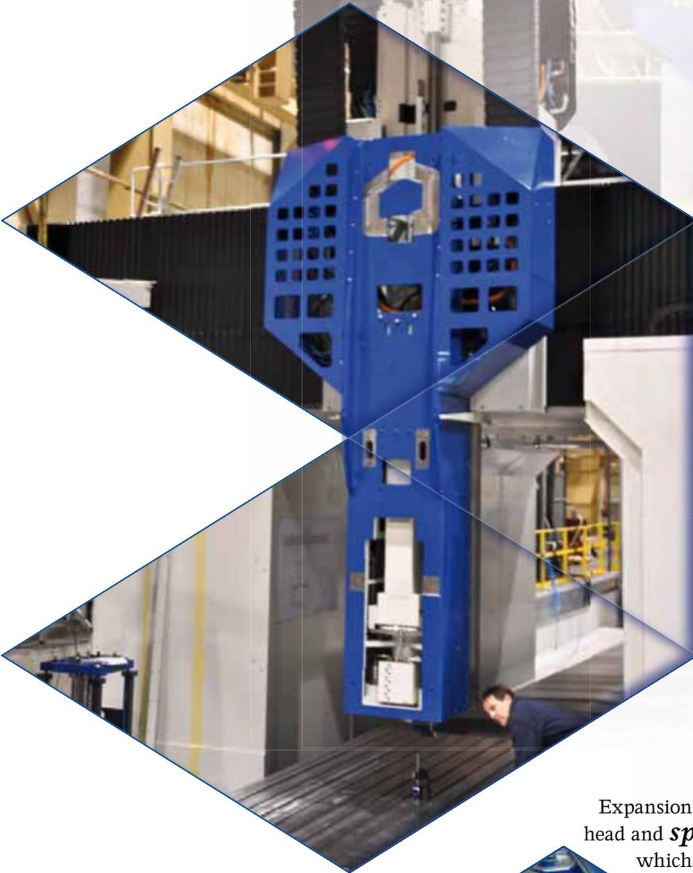
The compact design of the Z carriage can travel 2000mm, and can be equipped with either a gear-driven or motor spindle.
