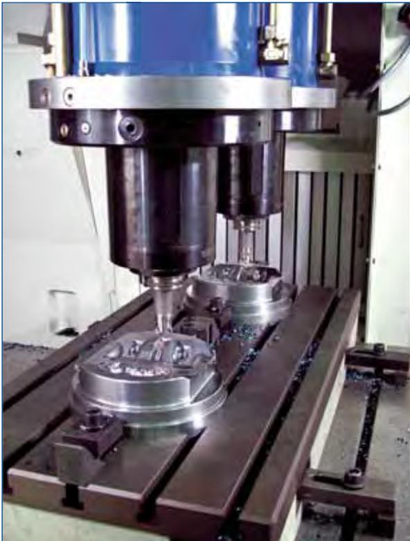
The MIKROMAT 8V, 8V 2S and 8V HSC are based on a dynamically and statically optimised design in portal style. The optimally-dimensioned machine bed and the rigid portal guarantee, in combination with the high-precision linear guidance system, long-term precision in the high accuracy range.
