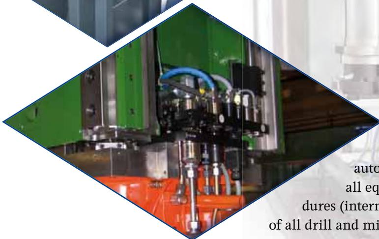
A central *power interface* with automatically-pluggable media coupling for all equipment functions and technical procedures (internal and external cooling). The direction of all drill and milling heads is configured automatically.
