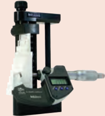
Micro checker 516-607 applicable gauge block sets 516-156, 516-157, 516-158
