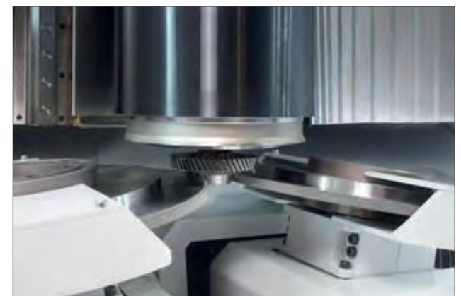
Synchronous O.D. grinding
