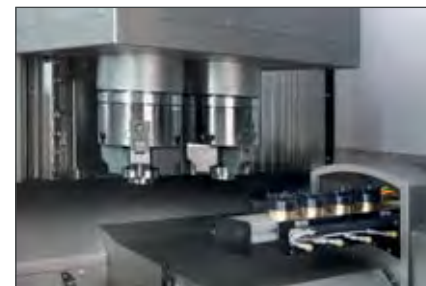
Linear loader: workpiece feeding
